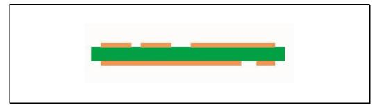
Figure 7.10 – PCB after Inner Layer Image Transfer
