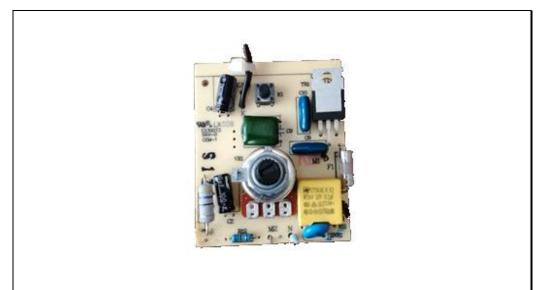
Figure 7.5 – A CEM Printed Circuit Assembly
