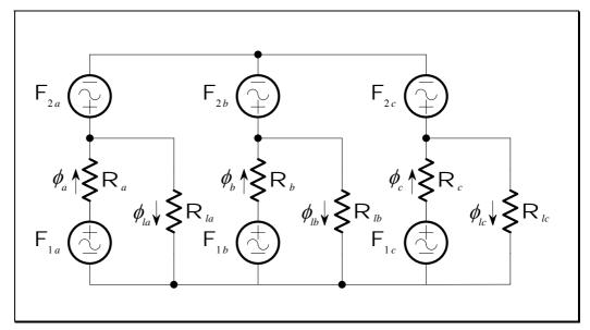
Figure 3.3 – Three-phase transformer magnetic equivalent circuit
