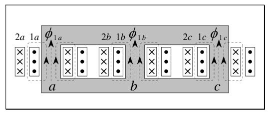
**Figure 3.2 – Three-phase transformer construction**
