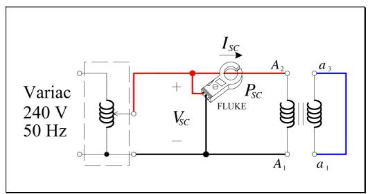
Figure 3.7 – Positive and negative sequence test circuit for leakage Z
