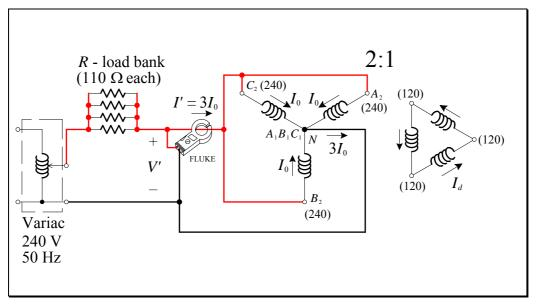
Figure 3.6 – Zero sequence test circuit for a star(earthed)- $\Delta$  transformer
