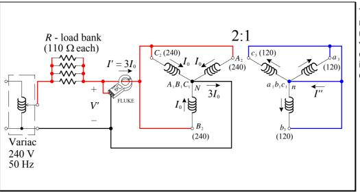
The Fluke clamp meter is used to measure the source voltage and any currents. The DMM is used to measure other voltages
