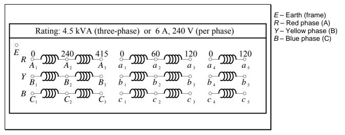
**Figure 3.1 – Three-phase transformer windings**
