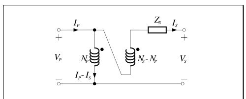
Figure 4.3 – Step-up autotransformer with leakage impedance
