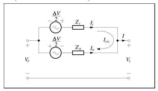
An equivalent circuit of two transformers in parallel is shown below:
