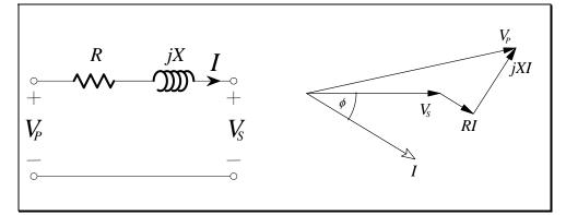
**Figure 4.4 – Transformer regulation**
