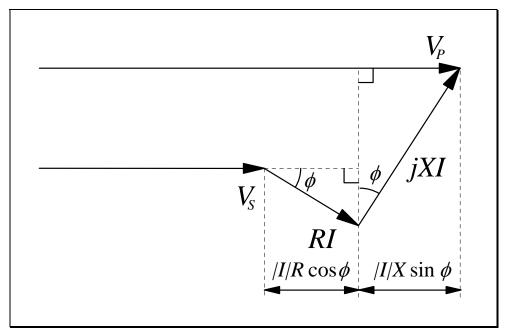
Figure 4.5 – Approximate transformer regulation
