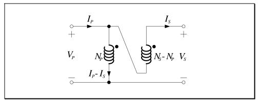
**Figure 4.2 – Step-up autotransformer**
